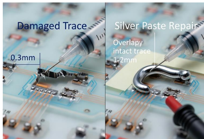
Figure 1. Damage Trace and Silver Paste Repair
